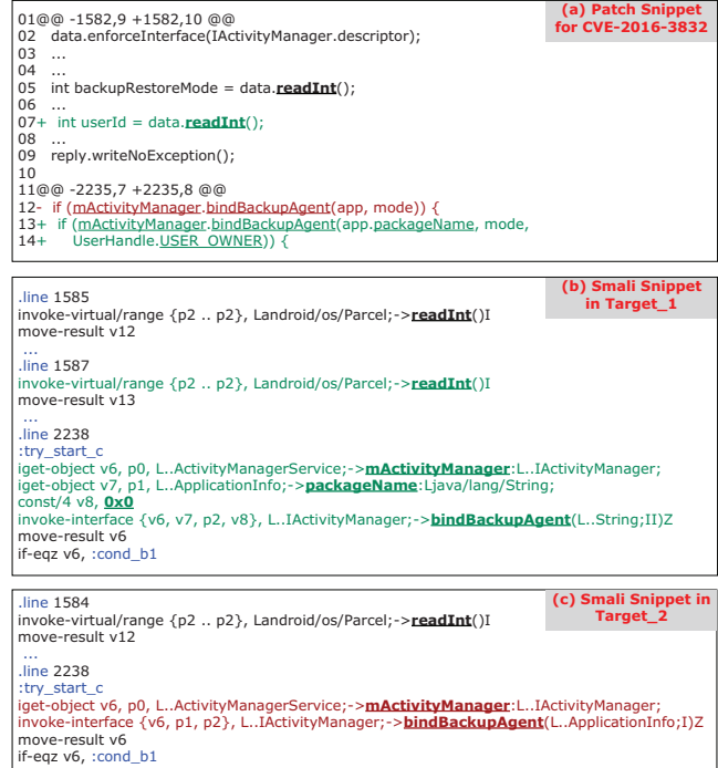
Figure 1: Patch Snippet for CVE-2016-3832 with code snippets from two target Java executables.
