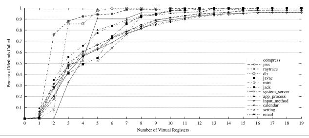
Figure 3. The percentage of invoked methods with varied number of virtual registers.
