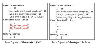
Figure 3: Path digests for pre-patch path <a,b,c,e,f,g> and post-patch path <br/>b,c,e,g>, using node g in Figure 2 as the anchor block.
